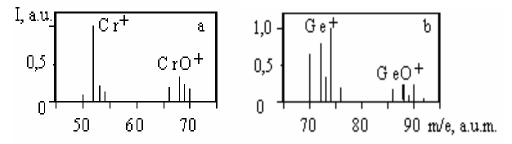
Fig. 1 – Mass spectrum of secondary ions films (a) Cr and (b) Ge of the side vacuum
